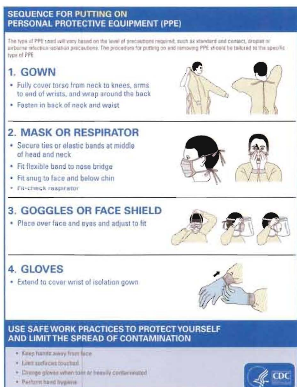
Fig. 5-18. Sequence for putting on personal protective equipment. (IMAGE REPRINTED FROM THE CDC'S WEBSITE, WWW.CDC.GOV/HAI/PDFS/PPE/PPE-SEQUENCE.PDF )
