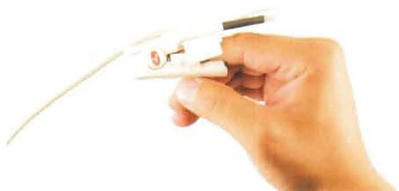
Fig. 14-16. A pulse oximeter sensor is usually clipped on a person's finger to measure the amount of oxygen in the blood, as well as pulse rate.
